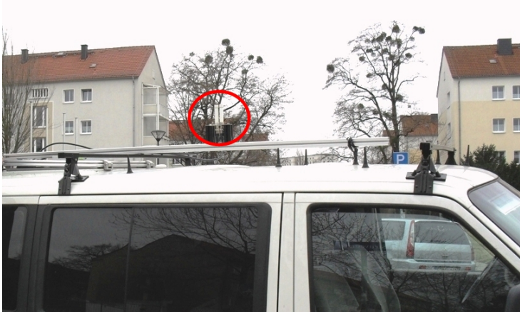
Figure 1.6. Two dipole antennas (inside the red circle) are mounted on a metal rod over the car roof. For more details, see Paper IV.
