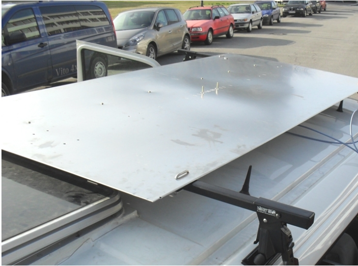
Figure 1.8. Two monopole antennas are mounted over a metal sheet to ensure that they experience similar fading. For more details, see Paper IV.
